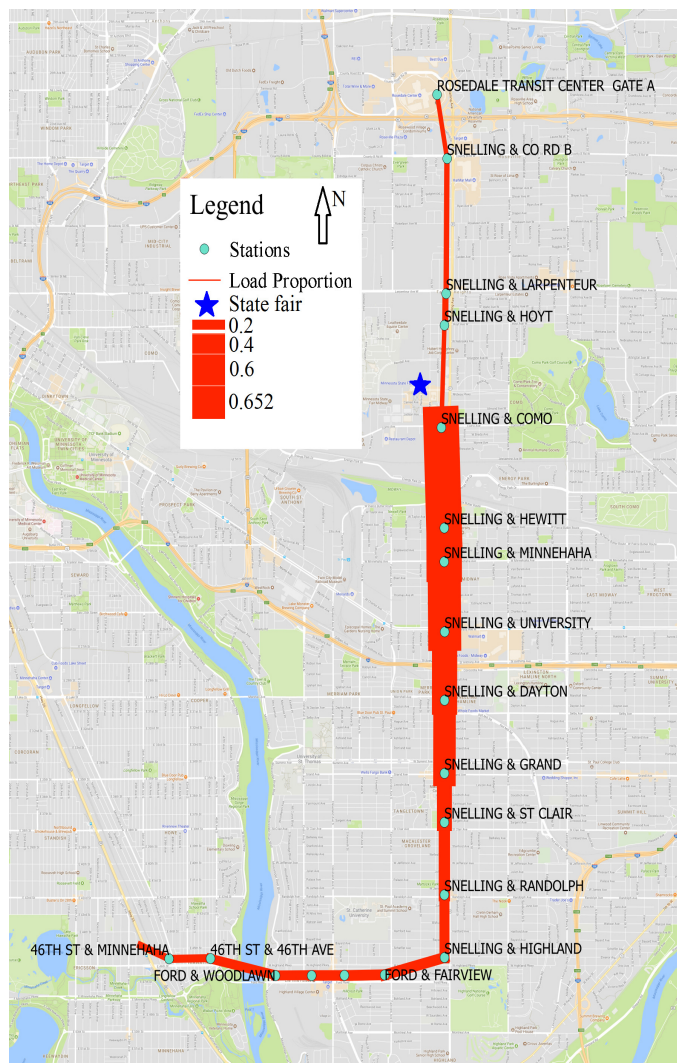
Fig. 5: Passenger load in southbound direction
